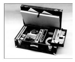
A fast-setting-cement kit, used to firmly attach the guide to the test part, is available as an accessory item.
